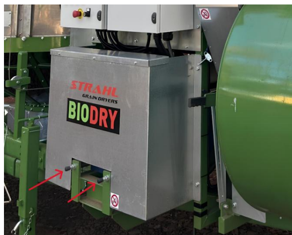
Figure 7.3 Threaded rods for electric motor disconnection.
