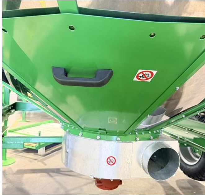
Figure 3.1 Silo cone access door
