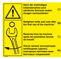
first After the all commissioning, connections screw must be tightened!
