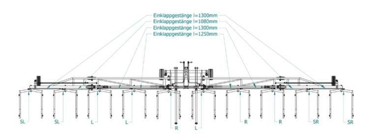
When assembling the heel harrow field beam, make sure that the left and right field beams are not mixed up.
