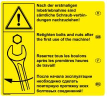
After the first commissioning, all screw connections must be tightened!
