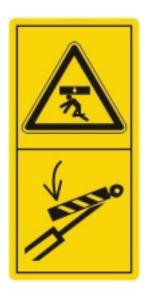
Stay clear of swinging range folding machine parts!
