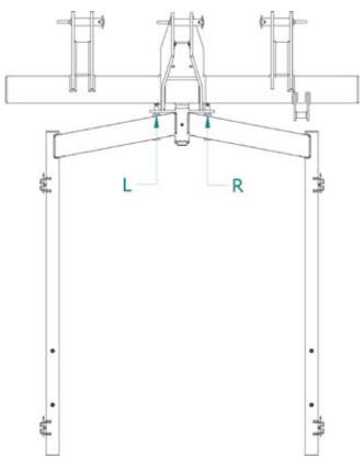
When assembling the heel harrow field beam, make sure that the left and right field beams are not mixed up.
