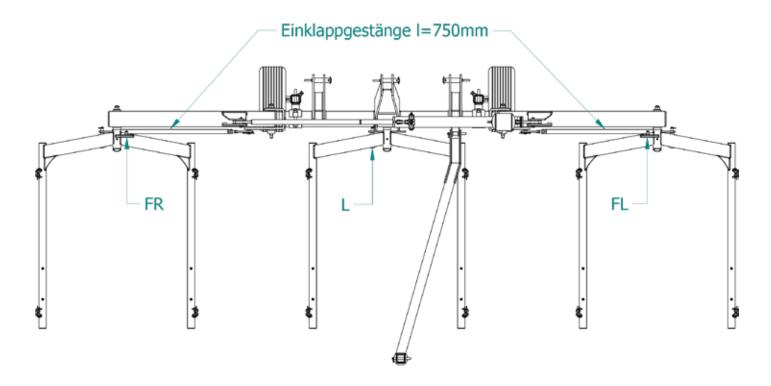
When assembling the heel harrow field beam, make sure that the left and right field beams are not mixed up.
