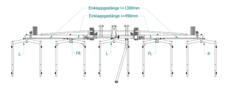
When assembling the heel harrow field beam, make sure that the left and right field beams are not mixed up.
