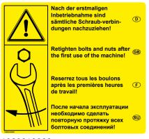
first After the commissioning, all connections screw must be tightened!
