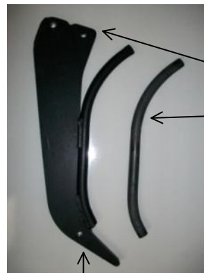
Standard Vari-Tilth Leg = 20mm thick
