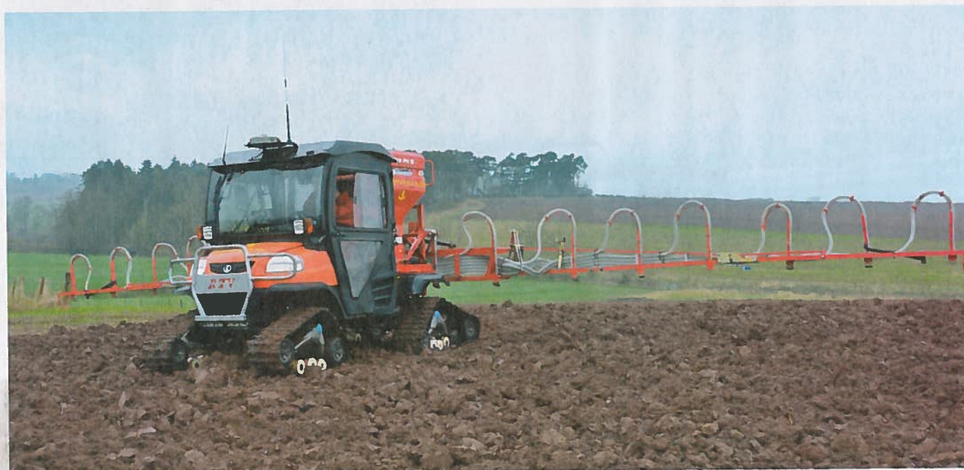
Kelso-based Crop Services runs its Kubota RTV on 30cm wide tracks fitted with beefed-up drive rollers to cope with the high torque loading and wet conditions
