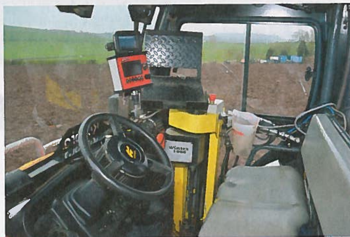
A control box for the 12m Opico Micro Pro is fitted in the air-conditioned cab
