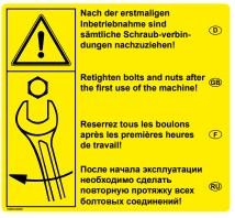
first After the all commissioning, connections screw must be tightened!
