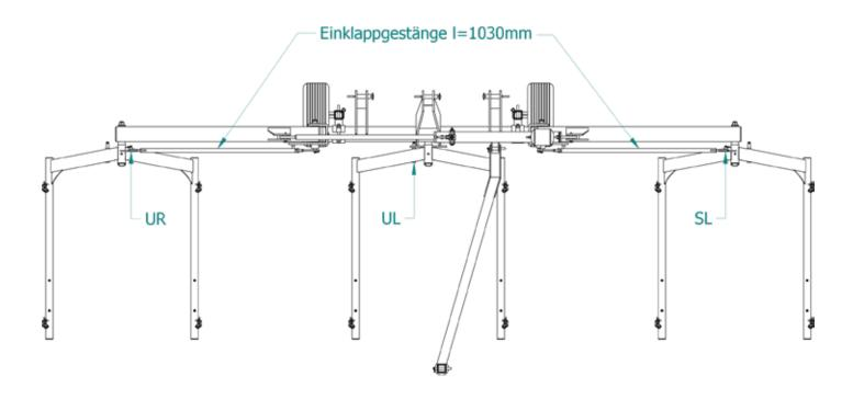
When assembling the heel harrow field beam, make sure that the left and right field beams are not mixed up.
