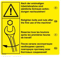
first After the commissioning, all connections screw must be tightened!
