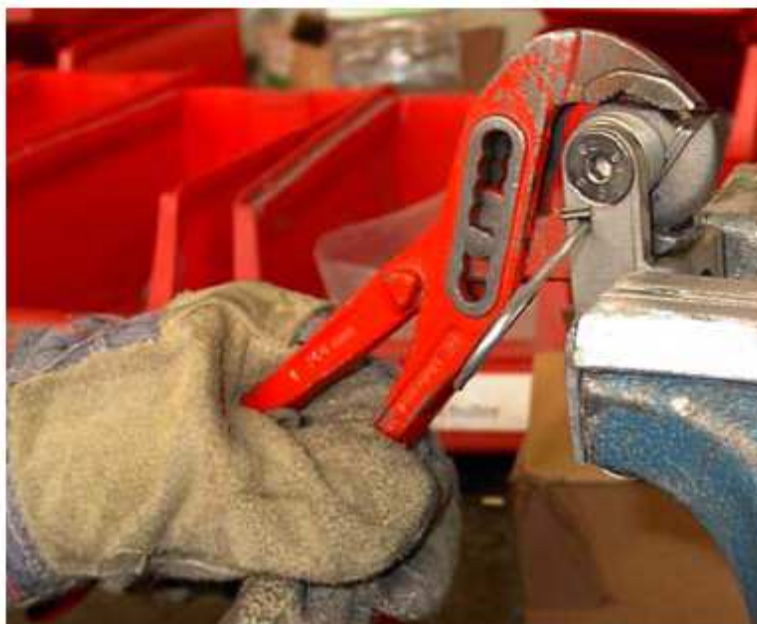
Figure 7 – Pre Loading Eccentric Adjuster
