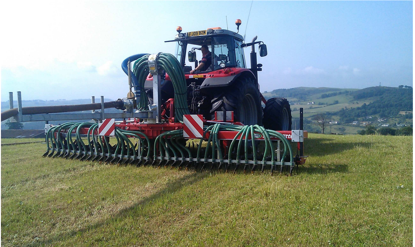
Figure 2 – OPICO 6m Sward Slitter c/w Slit Injector
