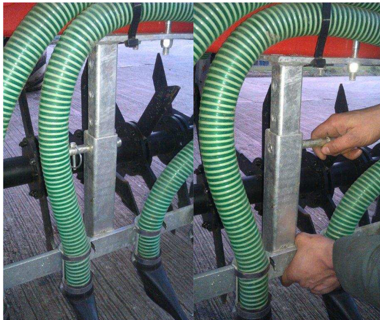
Figure 4 – Slit Injector coulter bar adjustment.
