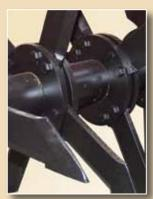
Blades are securely sandwiched in position from both sides using a steel ring which is fully welded to the axle, a second ring clamps the blades into position and secures them using bolts. This ensures secure fixing preventing loss of bolts and blades which cause havoc with grass harvest
