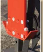
The protective skids on each axle mounting protect the axles by limiting the working depth of the machine, they also protect the bearings from ingress of soil. The angle of the axle can be altered to 5° to make the blades more aggressive.
