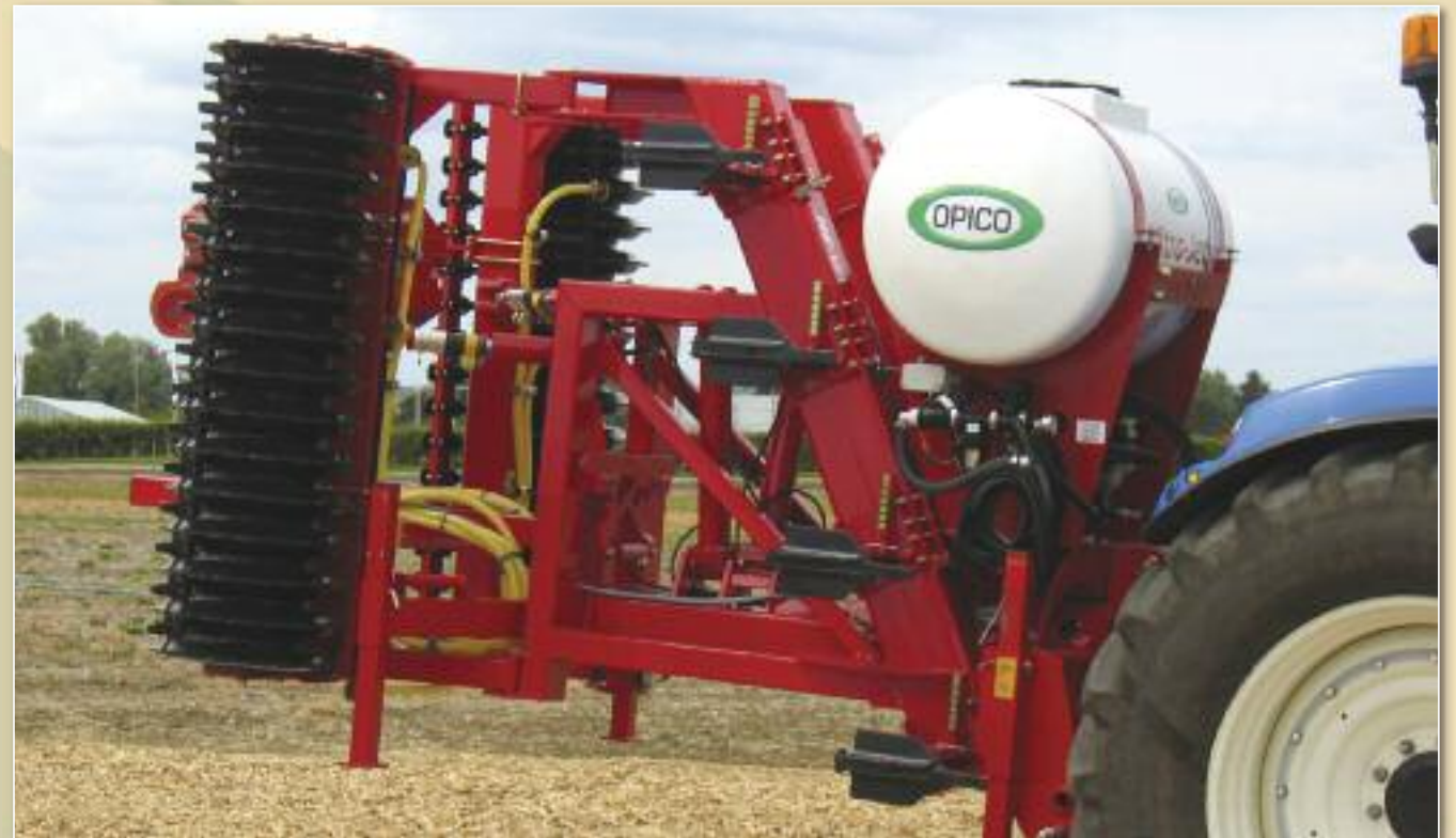
Integrated Nitro-Jet mounted on a 4m 7 Leg HE-VA Subsoiler with Variocast 8 Electronic Seeder
