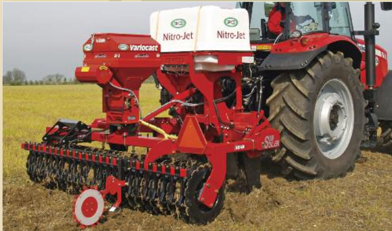
Integrated Nitro-Jet mounted on a 3m 5 Leg HE-VA Subsoiler with Variocast 8 Electronic Seeder
