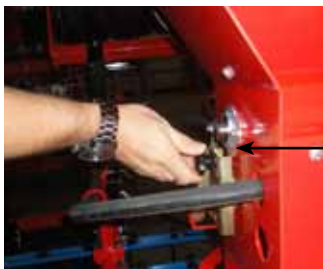
Opening the bearing support of the closing flap by thumbscrew
