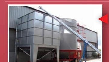
The pre store hopper can also be loaded directly by a materials handler if required, whichever way it is full by the time the previous load is finished
