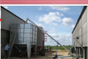
The pre storage hopper, which is matched to the size of the Dryer, is gradually loaded whilst the Dryer is at work on the previous load
