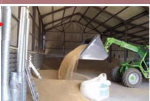
The reception pit can be loaded by a materials handler when a wet grain pile has built up and trailers are not coming in from the field
