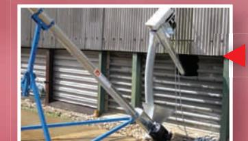
The transfer auger is then loaded from the undercover sunken reception pit
