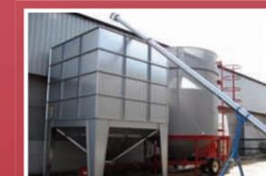
The pre store hopper can also be loaded directly by a materials handler if required, whichever way it is full by the time the previous load is finished
