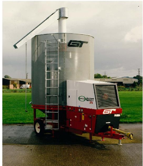
Supplied as standard with 33" custom-built, in-line centrifugal fan (74 dba). 8" diameter loading auger (50 ton an hour loading capacity). Full length 9ft 10" (3m) loading hopper. 60 ton an hour 12" diameter central auger. Centralised greaser location. Epoxy powder coated outside sheets. Adjustable screw jacks. Grain sampler, grain cleaner. Grain pressure splitter pelmet. LP gas fired burner. Grain Guard Monitor control system.
