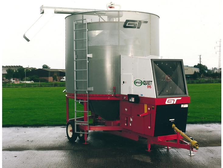
Supplied as standard with 38" custom-built, in-line centrifugal fan (74 dba). 8" diameter loading auger (50 ton an hour loading capacity). Full length 9ft 10" (3m) loading hopper. 60 ton an hour 12" diameter central auger. Centralised greaser location. Epoxy powder coated outside sheets. Adjustable jacks. Grain sampler, grain cleaner. Grain pressure splitter pelmet. LP gas fired burner. Control system: 575QF Push Button control - 595QF Grain Guard Monitor
