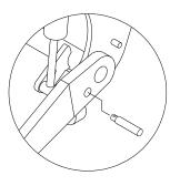
The lift arms are equipped with a shaft for floating position.
