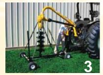
Step 3: Disconnect the digger from the tractor 3-pt. hitch.
