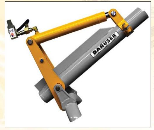
Down force kits are available to make difficult digging easier. The kits attach to all Danuser boomtype diggers without alteration and with the use of ordinary hand tools. They provide approximately 500 pounds of additional force to the auger point for easier penetration of hard or frozen ground.
