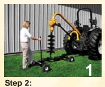
Attach the four ratchet straps, and disconnect the driveline or hydraulic hoses. Support the digger yoke with the yoke support assembly.
