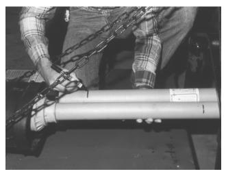
H. Hold driveline sections parallel to each other and check for minimum 6 inches (15cm) overlap. Figure 2-3). If driveline has been marked for cutting, overlap will be the distance between two marks. If driveline has less than minimum overlap, do not use. Contact authorized Bush Hog dealer.
