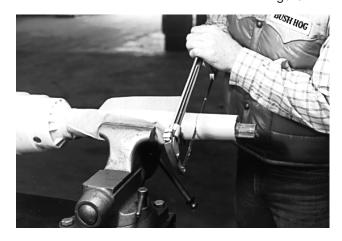
J. Using cut off section of shield as a guide, cut shaft the same amount. (Figure 2-5)
