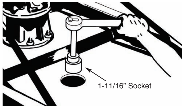
Figure 4-2 Blade Nut Removal
