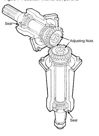
Figure 4-5 Tightening Bearings
