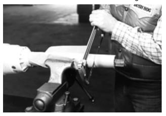
J. Using cut off section of shield as a guide, cut shaft the same amount. (Figure 2-6)
