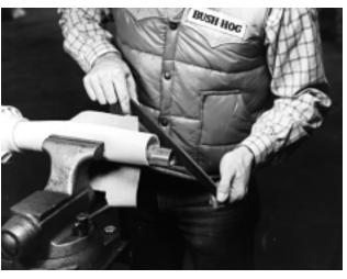
M. Apply multi-purpose grease to inside of outer (female) driveline section. Assemble driveline and install on tractor and cutter. Pull on each driveline section to be sure yokes lock into place. Make certain driveline shielding is in place and in good condition.
