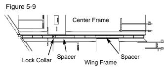
M. Place a 2-4 inch block under each center section front skid. Raise rear of center section until it is level and install stop collars on height adjustment cylinder to retain in this position.
