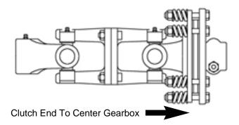
Q. Attach shield assembly to center gearbox using four 10mm x 25mm bolts, lockwashers and flatwashers. (Figure 5-13) Remove four bolts from power divider gearbox. Attach shield assembly to top of power divider gearbox using four 10mm x 50mm bolts (from bag of fasteners) lockwashers and flatwashers.
