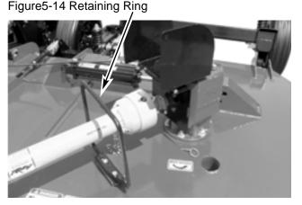
R. Attach U-joint retaining bracket to the mounting bracket welded to the deck of each wing in front of the gearbox input shaft. Secure with two 1/2" x 1-1/2" bolts, lockwashers and locknuts. (Figure 5-14)
