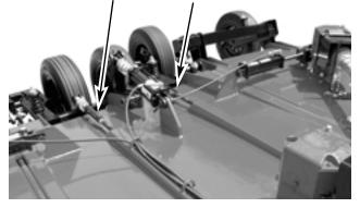
If you are cutting in dense material, operating cutter with the rear slightly higher than the front will allow an increased volume of cut material to exit from underneath cutter. This will decrease the cutter horsepower requirements.
