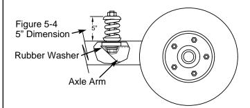
E .If the wing sections are equipped with single wheel option, the wheel should be assembled to the outside of the axle arms.
