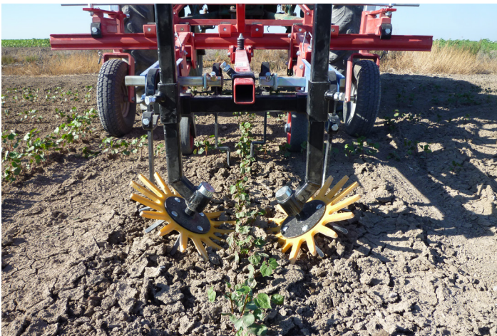
1.5m KULT Argus hoe with manual steer in a single row of beans complete with 370mm diameter yellow finger weeders and L blades.
