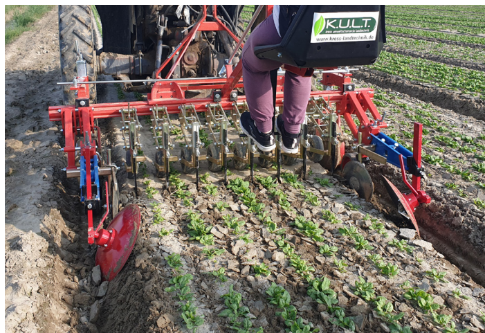
2m KULT Argus hoe with manual steer in spinach on raised beds with duo solo, inter-row weeding units and ridging discs.
