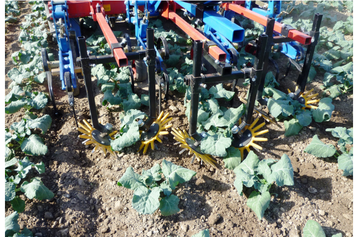
2m Hatzenbichler hoe with manual steer in rows of cabbage with 370mm diameter KULT finger weeders and S tines.
