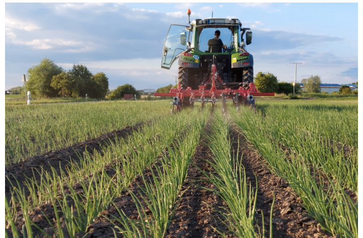
3m KULT Argus hoe using a PV frame with Tillett and Hague camera guidance in 30cm rows of onions with vibro spring tines.
