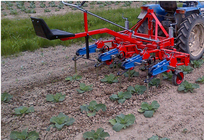
2.5 m KULT Argus hoe with manual steer in 3 rows of cabbage with vibro spring tines.
