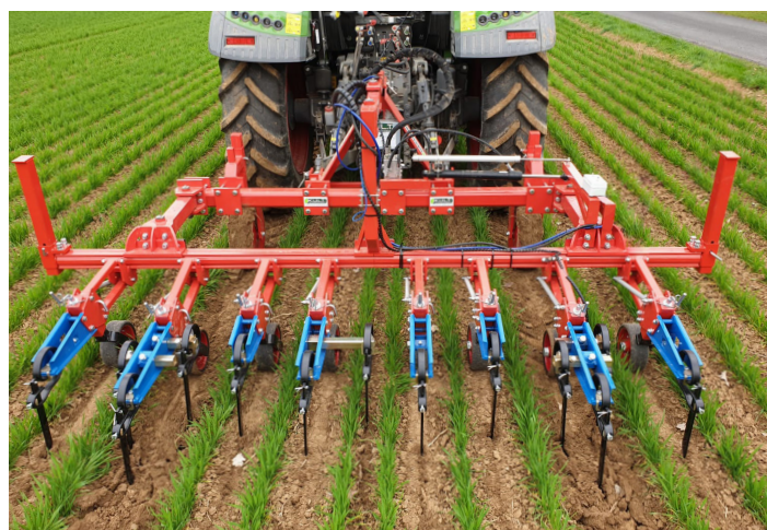
3m KULT Argus hoe with PV frame fitted with Tillett and Hague camera guidance in 25cm rows of wheat with vibro spring tines.
