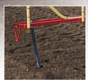
The plastic sway legs ensure a minimum boom height is maintained on undulating ground which prevents uneven application.
