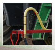
Vertical pipe above the outlet ensures the micro-granules hit the centre of the distribution plate and spread evenly.
