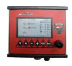
The control box allows setting and adjustment on the move, records the area that has been covered and keeps track of the amount that has been spread. A speed sensing motor constantly checks metering roller speed and this is adjusted by the computer control box to give you a constant rate.
