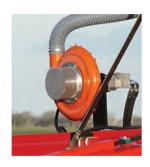
A hydraulic fan provides ample airflow to deliver the granules to the outlets and create a double overlapping spread pattern.
