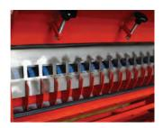
The stainless steel baffle ensures even airflow within the metering system and ensures that only one outlet is fed from each metering segment.
