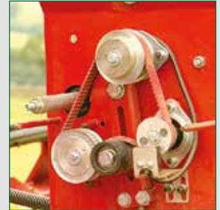
A toothed non-slip belt is used for positive drive and all seeders are fitted with a drive belt sensor. The toothed belt also drives the agitator inside the hopper to maintain a steady flow. The agitator can be simply engaged or disengaged as required for delicate seed types.
