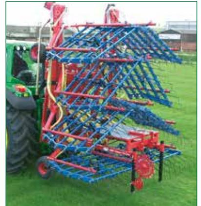
When in transport position, the hydraulic folding models fold to between 2.5m and 3m dependent on the model of grass harrow. This allows easy transportation on the road and through narrow gateways.
