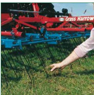
The Grass Harrow's 7 or 8mm spring tines are able to penetrate even the hardest of ground, ripping out dead thatch and opening up the soil surface allowing air into the root zone to stimulate growth.
