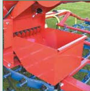
All machines are calibrated by removing the metering roller cover and using the calibration tray.
