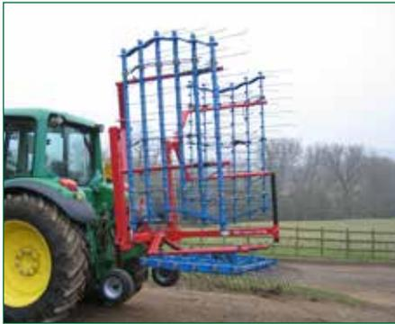
Working widths range from a very handy 1.5m to 12.4m. There are rigid and hydraulic folding units with a choice of 7mm or 8mm tines.
