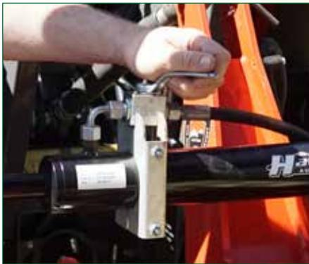
Hydraulic cylinder with lock to ensure safety during road transport.
