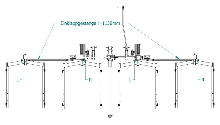
When assembling the heel harrow field beam, make sure that the left and right field beams are not mixed up.
