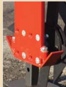
The protective skids on each axle mounting protect the axles by limiting the working depth of the machine, they also protect the bearings from ingress of soil. The angle of the axle can be altered to 5° to make the blades more aggressive.
