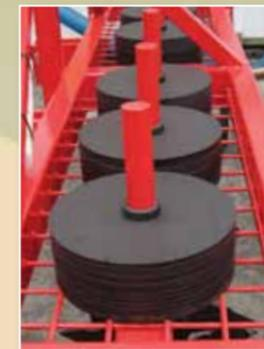
All machines come with a weight rack fitted as standard, optional weight spindles and disc sets are available for use in hard conditions. Each spindle and disc set consists of 1 x spindle + a set of disc weights, weighing approximately 90kg in total.
