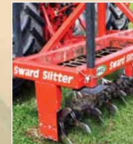
All Sward Slitter's come with heavy duty, robust frames for added durability and longevity. The frame also adds some extra weight that is needed in the dryer months ensuring the blades penetrate the ground fully, improving drainage and removing surface compaction.
