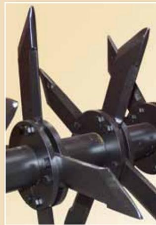
The oil hardened boron steel points incorporate a chamfered trailing edge. This limits the turf damage when each 210mm knife comes out of the soil, so leaving a clean finish. OPICO Slitters incorporate more blades per m than many machines ensuring optimum aeration effect.
