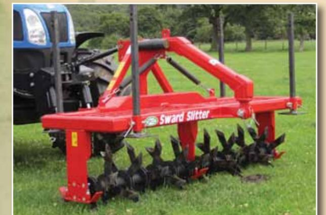
As an alternative to the rear mounted Slitters OPICO also offer 2.5m or 3m front mounted Slitters. These enable the Slitter to be used in combination with additional rear equipment such as a OPICO Sward Lifter. Mounted on a floating headstock the Slitter is effectively pulled down the field allowing it to accurately follow the ground contours.
