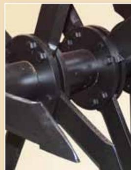
Blades are securely sandwiched in position from both sides using a steel ring which is fully welded to the axle, a second ring clamps the blades into position and secures them using bolts. This ensures secure fixing preventing loss of bolts and blades which cause havoc with grass harvest machinery.
