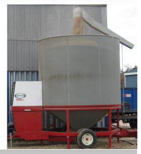
Supplied as standard with 32" axial fan (102 dba). Push button control system with fault indicating light panel. 8" diameter loading auger (50 ton an hour loading capacity). Full length 9ft 10" (3m) loading hopper. 60 ton an hour 12" diameter central auger. Centralised greaser location. Epoxy powder coated outside sheets. Adjustable jacks. Grain sampler , grain cleaner. Grain pressure splitter pelmet. LP gas fired burner.
