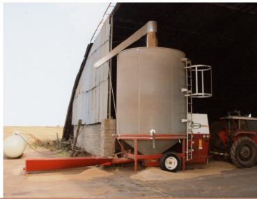
Supplied as standard with 26" axial fan (102 dba). 8" diameter loading auger (50 ton an hour loading capacity). Full length 9ft 10" (3m) loading hopper. 60 ton an hour 12" diameter central auger. Centralised greaser location. Epoxy powder coated outside sheets. Adjustable jacks. Grain sampler, grain cleaner, grain pressure splitter pelmet. LP gas fired burner. Control system: Push Button control with fault indicating light panel.
