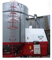
Electric drive requires 3-phase, 63 amp supply. Supply line to include 3-phases, earth and neutral on a dedicated circuit via residual current device and should be fitted by a qualified electrician.
