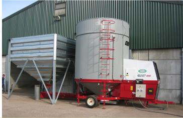
Supplied as standard with 38" custom built, in line centrifugal fan (74 dba). Unique self diagnostic electronic Grain Guard control. Centralised greaser location. 60 ton an hour 12" diameter central auger 8" diameter loading auger with full length, 9ft 10" (3m) loading hopper (50 ton an hour loading capacity). LP Gas fired burner. Epoxy powder coated outside sheets. Adjustable jacks, 4 tyres, grain sampler. Horizontal discharge auger. 3-phase electric drive.
