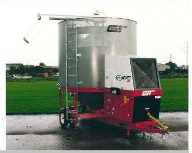
Supplied as standard with 38" custom-built, in-line centrifugal fan (74 dba). 8" diameter loading auger (50 ton an hour loading capacity). Full length 9ft 10" (3m) loading hopper. 60 ton an hour 12" diameter central auger. Centralised greaser location. Epoxy powder coated outside sheets. Adjustable jacks. Grain sampler , grain cleaner. Grain pressure splitter pelmet. LP gas fired burner. Control system: 575QF Push Button control - 595QF Grain Guard Monitor
