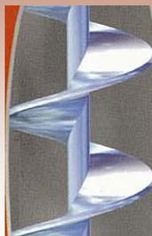
The 12" central auger continually circulates the grain in the dryer at 60 tonnes an hour. It's low 270 rpm handles the grain gently and the heavy duty fighting is built to stand the workload.
