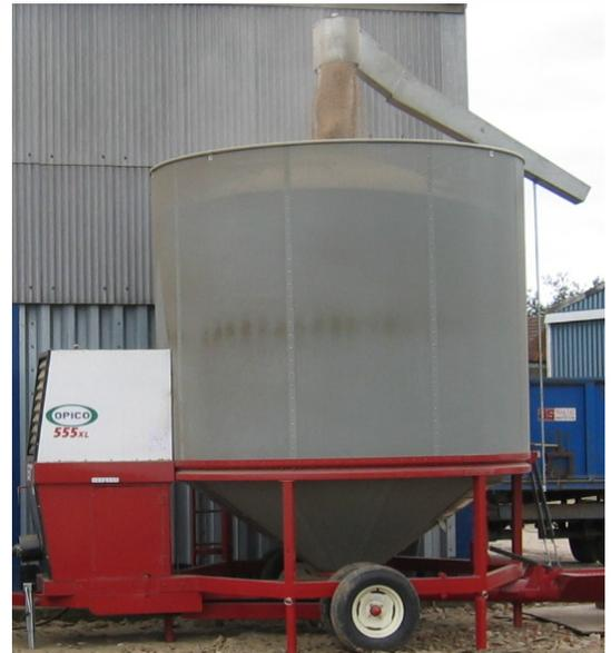
Supplied as standard with 32" axial fan (102 dba). Push button control system with fault indicating light panel. 8" diameter loading auger (50 ton an hour loading capacity). Full length 9ft 10" (3m) loading hopper. 60 ton an hour 12" diameter central auger. Centralised greaser location. Epoxy powder coated outside sheets. Adjustable jacks. Grain sampler, grain cleaner. Grain pressure splitter pelmet. LP gas fired burner.
