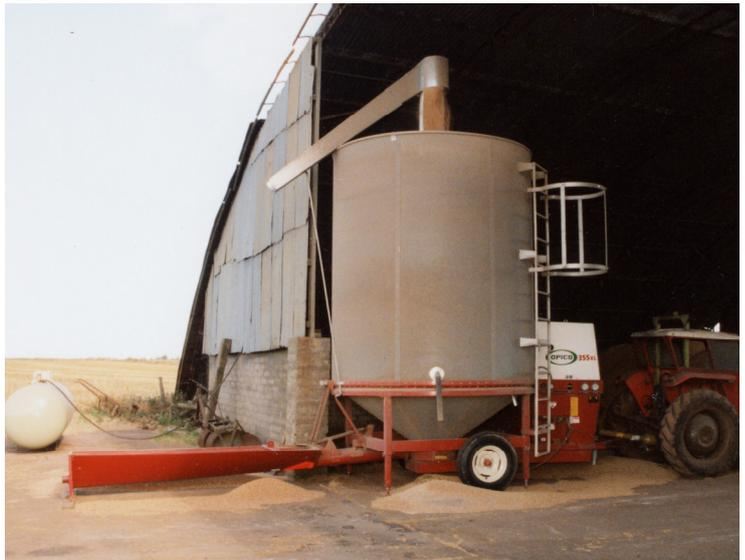
Supplied as standard with 26" axial fan (102 dba). 8" diameter loading auger (50 ton an hour loading capacity). Full length 9ft 10" (3m) loading hopper. 60 ton an hour 12" diameter central auger. Centralised greaser location. Epoxy powder coated outside sheets. Adjustable jacks. Grain sampler, grain cleaner, grain pressure splitter pelmet. LP gas fired burner. Control system: Push Button control with fault indicating light panel.
